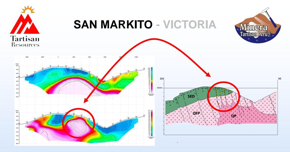
IP chargeability target coincident with breccia/stockwork zone at San Markito (L 1425 N shown)
